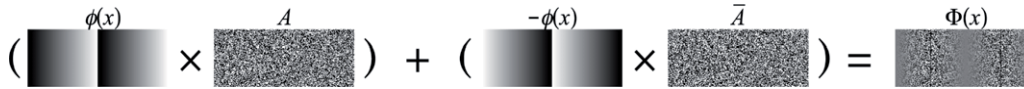
Figure 1. Scheme of the technique used to generate a multiplexed duplicator with random binary amplitude masks. \pm\phi(x) represent the two opposite signed linear phases yielding the two diffraction orders; A and \bar{A} represent two complementary binary random amplitude masks.
