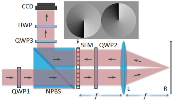
Fig. 1. Double pass system to generate generic  $q$ -plates.
